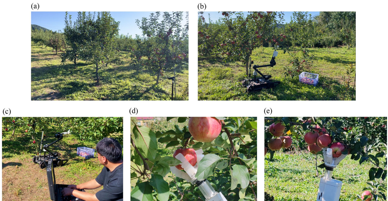
FIGURE 11 | Field trials and demonstration of the harvesting system. (a and b) Field trials conducted in a commercial apple orchard in Northeast China. (c) Field testing scenario with a robotic platform featuring an arm equipped with a soft gripper and remote control. (d) A video frame showing the soft gripper successfully picking an apple. (e) Examples of harvest failures caused by over-dense apple distribution and grasping interference. [Color figure can be viewed at wileyonlinelibrary.com ]
